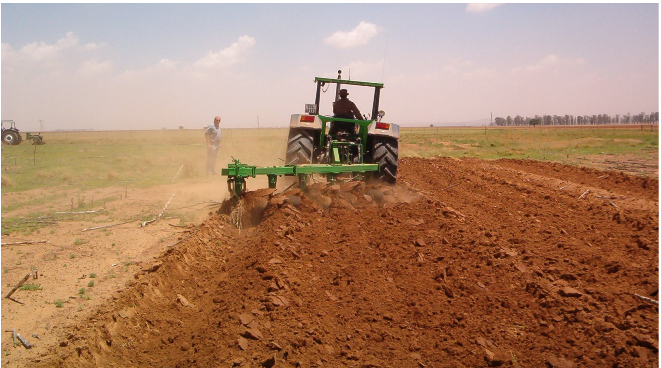
Modern tractor ploughing in South Africa. This plough has five non-reversible mouldboards. The fifth, empty furrow on the left may be filled by the first furrow of the next pass.
